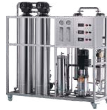
One stage RO pure water equipment
